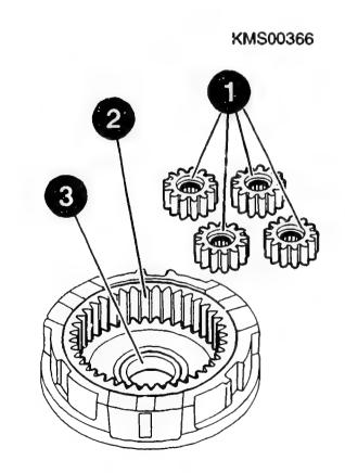
Checking planetary gear train
